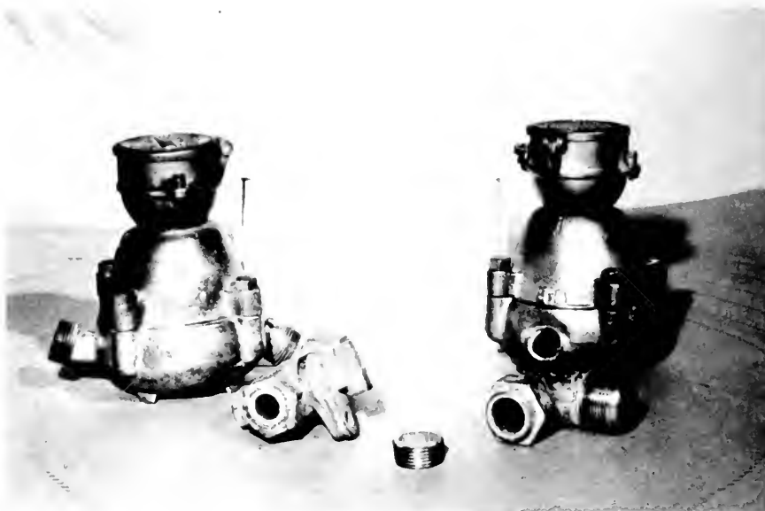
Photo 17. Water meters broken in earthquake. Los Angeles Department of Water and Power photo.
